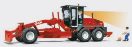
The O&K grader cab is a model of ergonomics. The operator' station is positioned for maximum visibility all-round through large, tinted windows to the front, the sides, and also right down to the ground. Even when seated, the operator has full view of both mouldboard ends. When reversing, the rounded tail-end allows excellent and safe visibility of any persons or objects within the machine's proximity.
