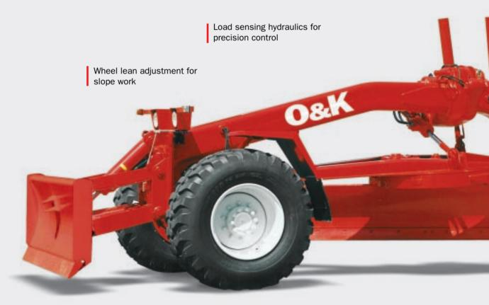
All-wheel drive with Electronic Drive Control for optimum traction on difficult terrain
