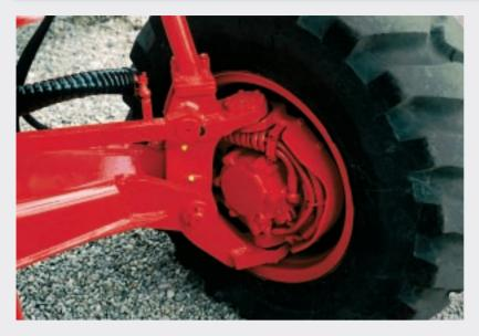
On the all-wheel drive model, the front wheels are driven by a swashplate pump and hub-mounted motors. Electronic drive control EDCV uses a differential lock to match oil volume and hence the front-wheel speed automatically to that of the rear wheels.
