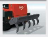
A front blade and rear ripper make the F 156/A grader from 0&K even more versatile.
